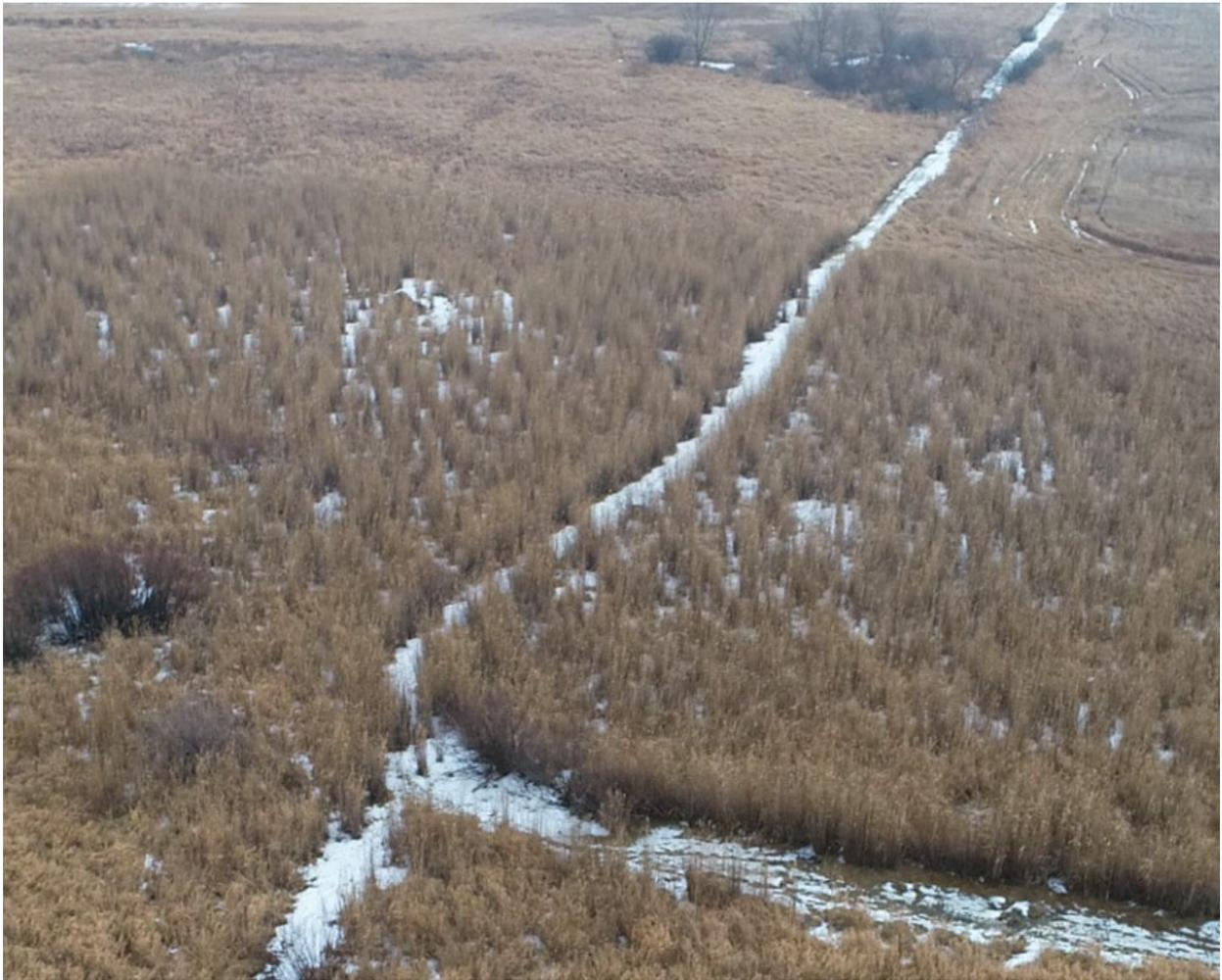
This area represents the legal beginning of the ditch. The channel in this area is defined has good width. There is vegetation in and around the channel with the ditch running through Type 3 wetlands.
