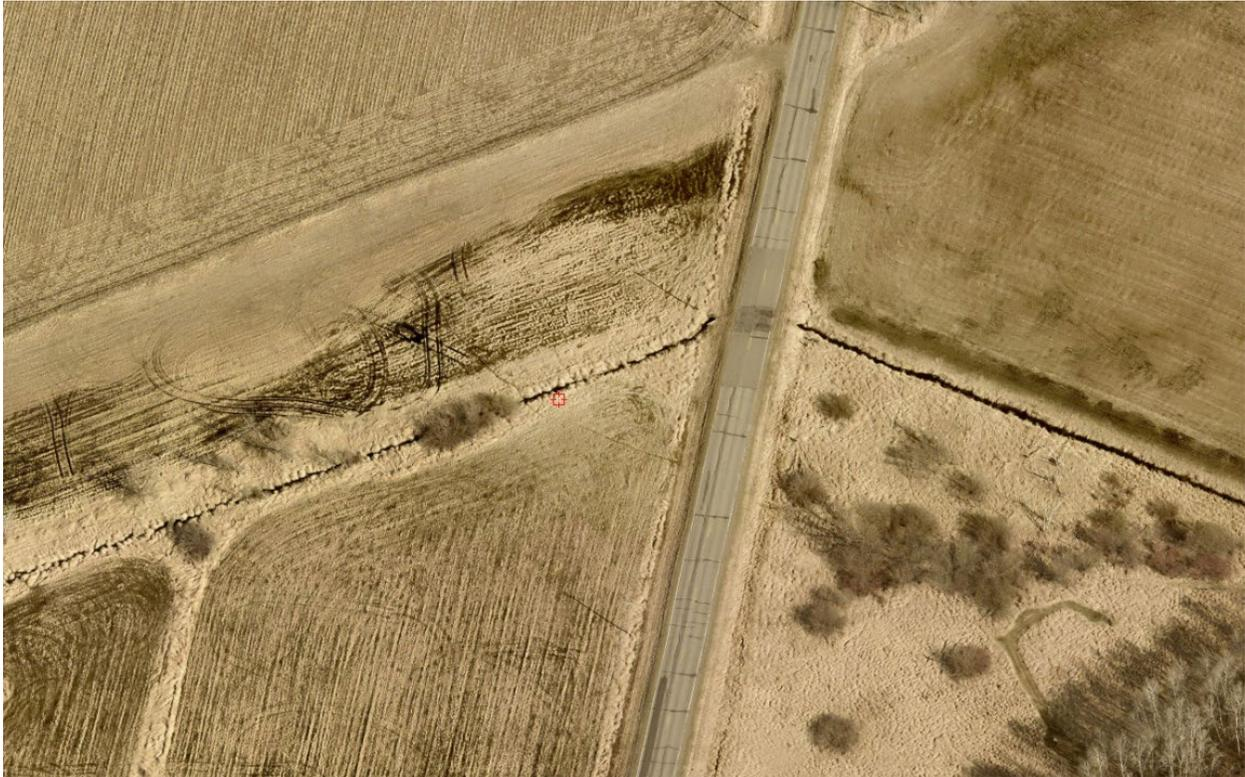
The ditch west of Co Rd 137 has vegetation constriction compared to the east side but is generally free of obstruction.
